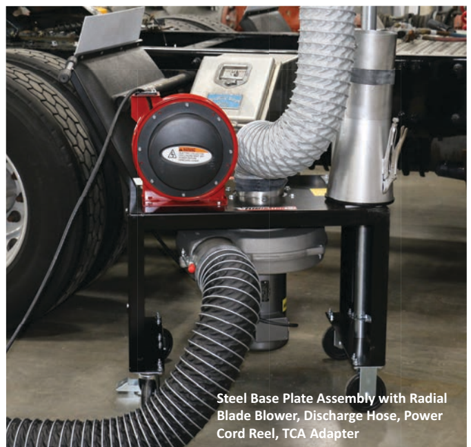
Standard Eliminator with 45-degree Stack Nozzle for Truck Application
